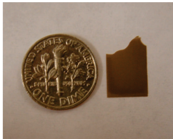
Figure 1. Digital image of a freestanding TiO 2 nanotube membrane in brown (right). The lateral dimension of the membrane is comparable to a dime shown in the left.
